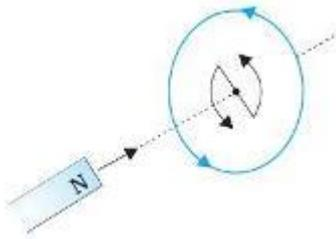
When we withdraw the magnet away from the coil, its upper face acquires south polarity. Now the work done is against the force of attraction.
