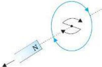
When the magnet is moved, the number of magnetic lines of force linking the coil changes, which causes an induced current to flow through the coil. The direction of the induced current, according to Lenz's law is always to oppose the motion of the magnet. The work done in moving the magnet is converted into electrical energy. This energy is dissipated as heat energy in the coil.
