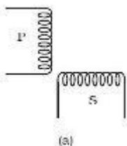
When a current is passed through coil P, the magnetic flux linked with S is small and hence, the coefficient of mutual induction between the two coils is small.
