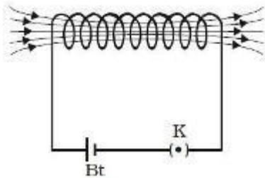
On pressing the key, the current through the coil increases to a maximum value and correspondingly the magnetic flux linked with the coil also increases. An induced current flows through the coil which according to Lenz's law opposes the further growth of current in the coil.
