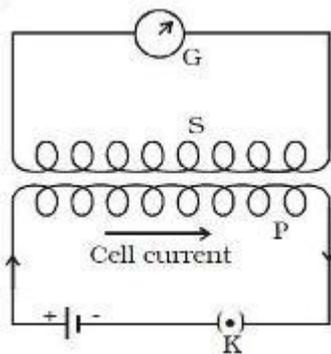
Whenever there is a change in the magnetic flux linked with a coil, there is also a change of flux linked with the neighbouring coil, producing an induced emf in the second coil.
