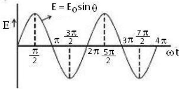
As the armature completes  $\nu$  rotations in one second, alternating current of frequency  $\nu$  cycles per second is produced.
