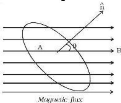
If  $\theta$  is the angle between the direction of the field and normal to the area, then
