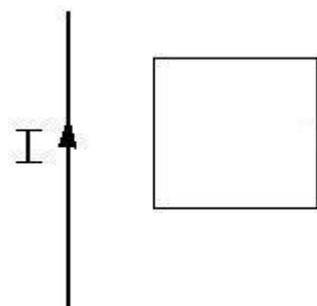
Figure shows a conducting loop placed near a long, straight wire carrying a current  $I$  as shown. The direction of magnetic field will be going inside the paper
