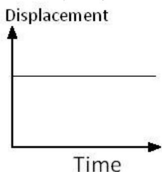
Slope of straight line (representing instantaneous velocity) is zero.
