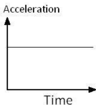
The area enclosed by acceleration - time graph for the body for the given time gives change in velocity of the body for given time
