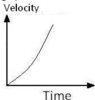
The slope of the graph increases with time. or instantaneous acceleration increases with time
