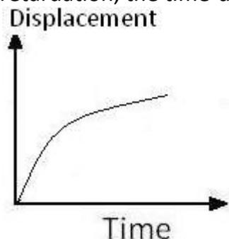
The slope of time-displacement curve ( i.e. instantaneous velocity) decreases with time.
