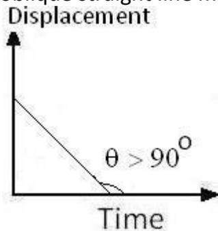
Displacement of the body decreases with time with respect to the reference point, till it becomes zero
