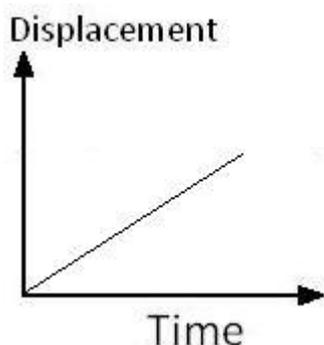
Greater is the slope of straight line higher is the velocity
