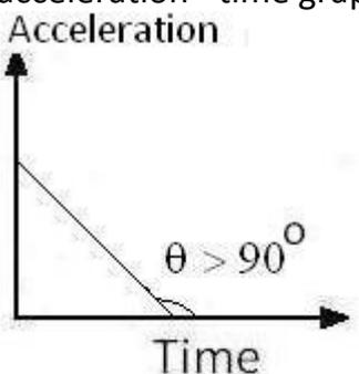
The body is moving with negative acceleration and slope of straight line makes an angle  $\theta > 90^\circ$  with time axis. Or slope of the line is negative
