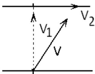
The boat should go along the direction, perpendicular to the direction of river flow. then the boat will be going along the direction of resultant velocity  $\vec{v}$  of velocity of boat  $\vec{v}_1$  and velocity of flow of river  $\vec{v}_2$ . If  $\vec{v}$  making an angle  $\theta$  with the direction of  $\vec{v}_1$ , If  $S$  is the width of river and time  $t$  is time of crossing then
