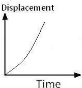
The slope of time-displacement curve increases with time or velocity is increasing with time
