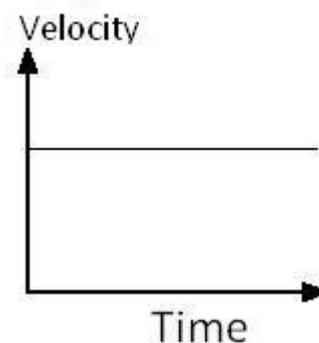
The slope of the graph , representing the instantaneous acceleration is zero
